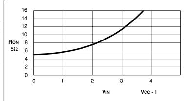
Figure 2. QuickSwitch ON Resistance vs. VIN
