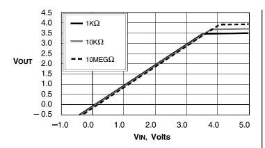
Figure 3. Typical Vout vs. VIN for Various Loads
