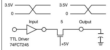
Figure 6. Bus Switch Operation
