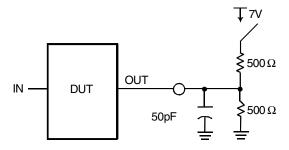
Figure 9. AC Test Circuit for 5V Products
