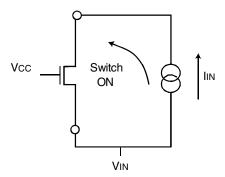
Figure 8. QuickSwitch R<sub>ON</sub> Measurement
