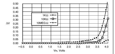
Figure 4. Typical Voltage Drop vs. VIN
